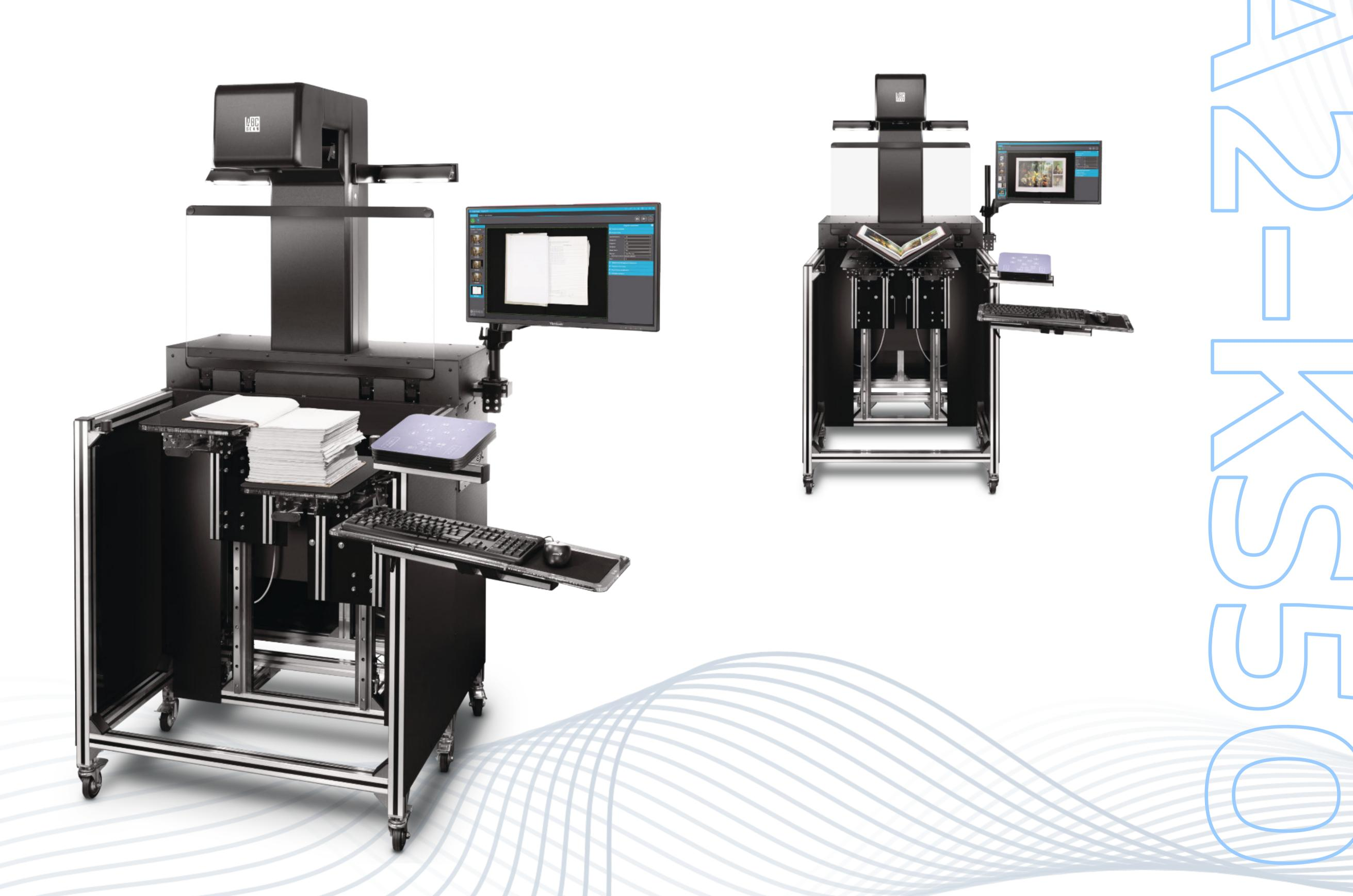
The main feature of ElarScan A2–KS50 is the integrated DIN A2 flip–up flat glass with electromagnetic locks and electronic control from the front panel. The scanner supports semi–automatic mode, operator can only turn the page and close the glass, no any other action. Scan starts when the glass is closed and glass opens immediately after the scanning is completed.
