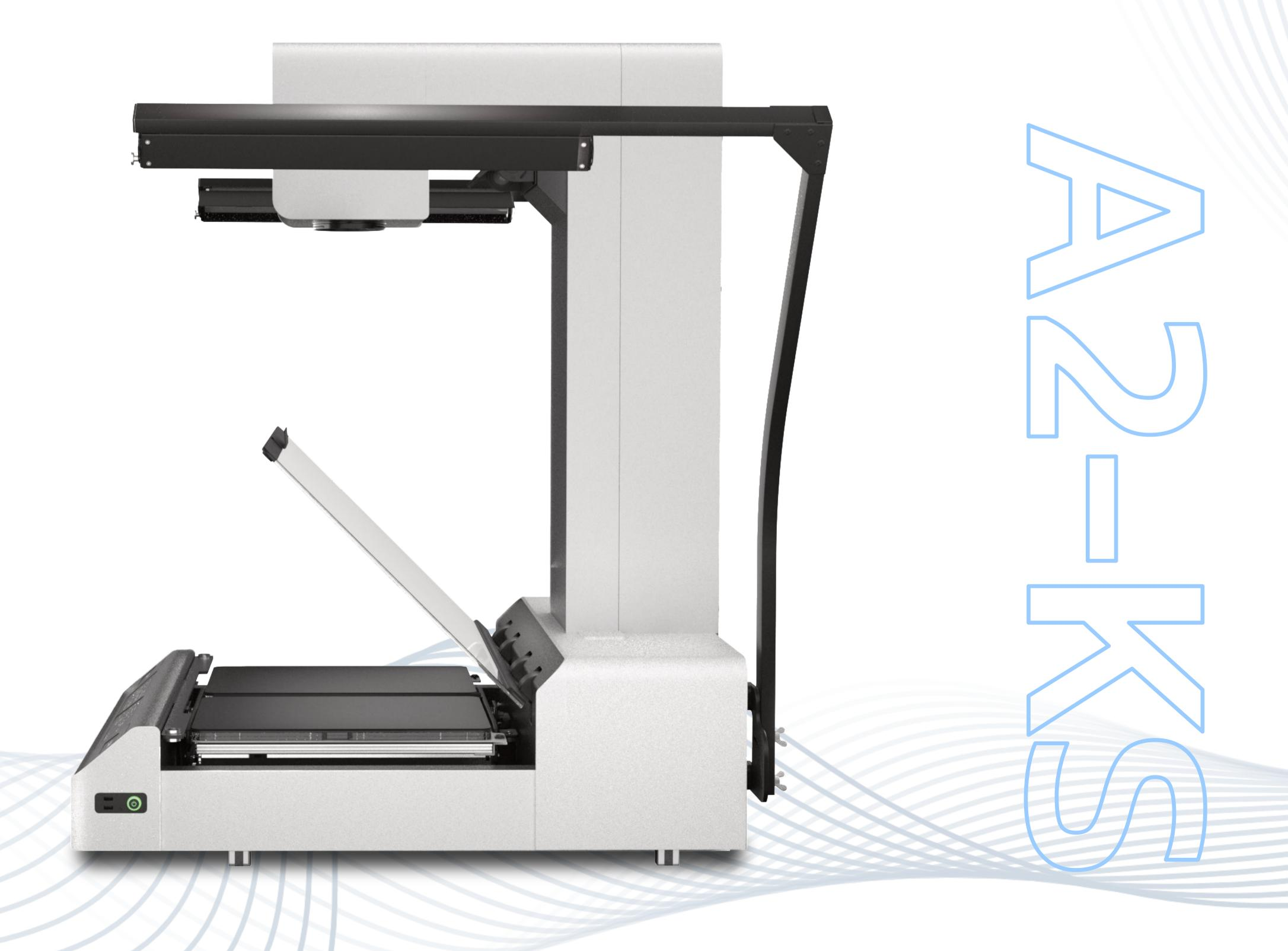
The main feature of ElarScan A2–KS is the integrated DIN A2 flip–up flat glass with electromagnetic locks and electronic control from the front panel. The scanner supports semi–automatic mode, operator can only turn the page and close the glass, no any other action. Scan starts when the glass is closed and glass opens immediately after the scanning is completed.
